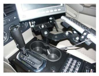
Final assembly of C-TCB-7 (w/ C-TCB-MAK option), a C-VS-1600-EXPL, and an MW-800 computer system
